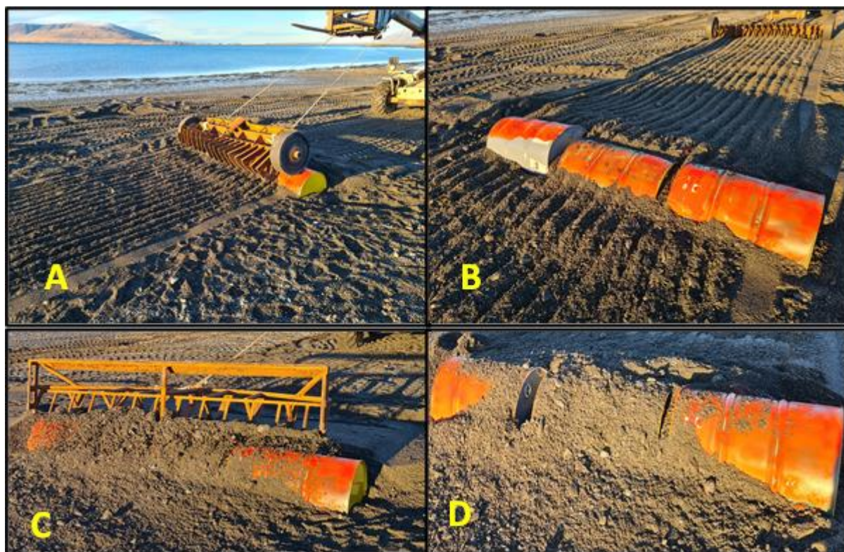
Figure 7-6. Dredges were towed at similar angle and speed as would be during actual fishing. Plate A shows the Berg's gear impacting the obstacle and plate B moments after. Plate C and D show same event for the Drag gear.
