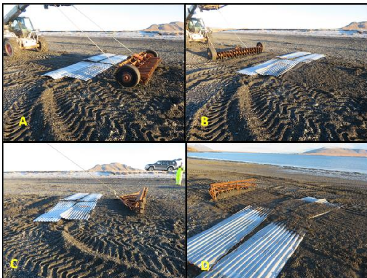
Figure 7-7. Corrugated steel plates were used to demonstrate how easily the dredges would run over flat obstacles. Plates A and B show the impact of the Berg's gear and plates C and D that of the Drag gear.
